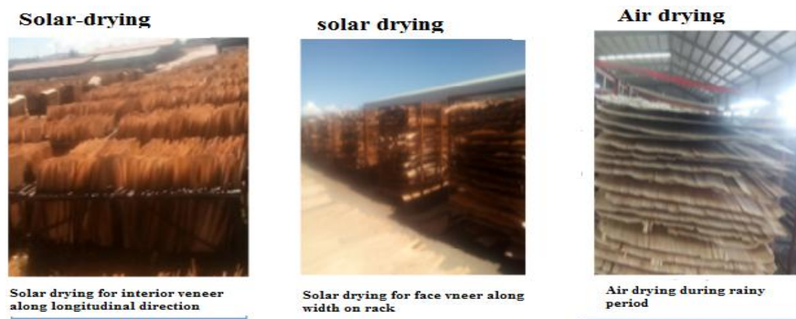
Figure 5. Veneer drying system and information
