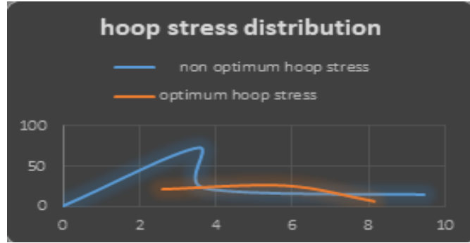
Figure 14. Thickness versus hoop stress graph
