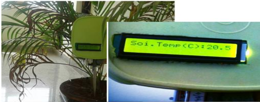
Figure 13. Application of the fabricated thermometer in real-time soil temperature monitoring in agriculture
