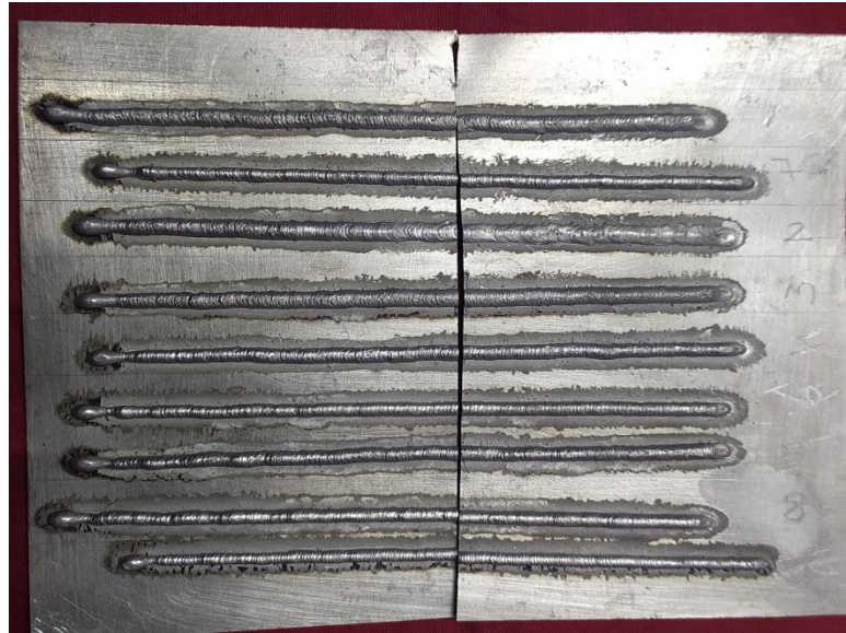
Figure 5. Cold Metal Transfer Welding
