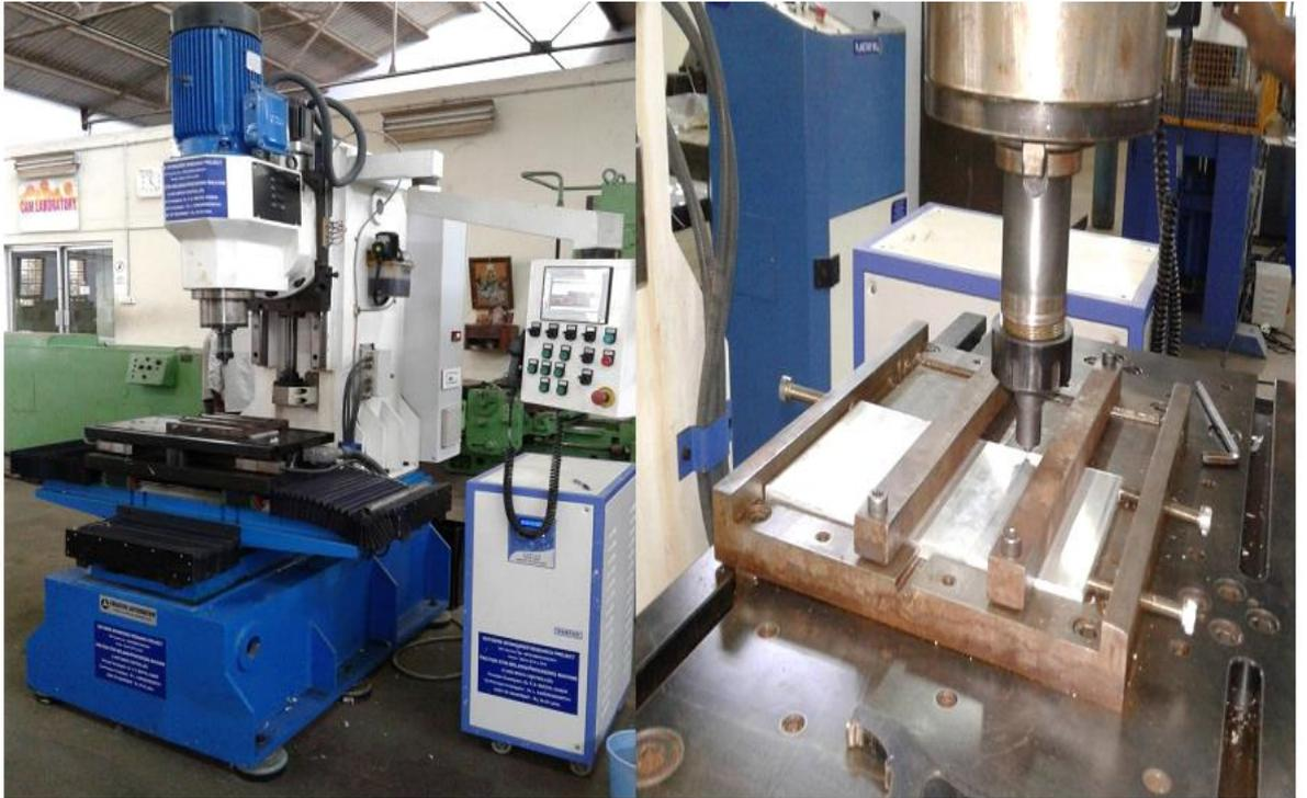
Figure 3 Friction stir welding setup
