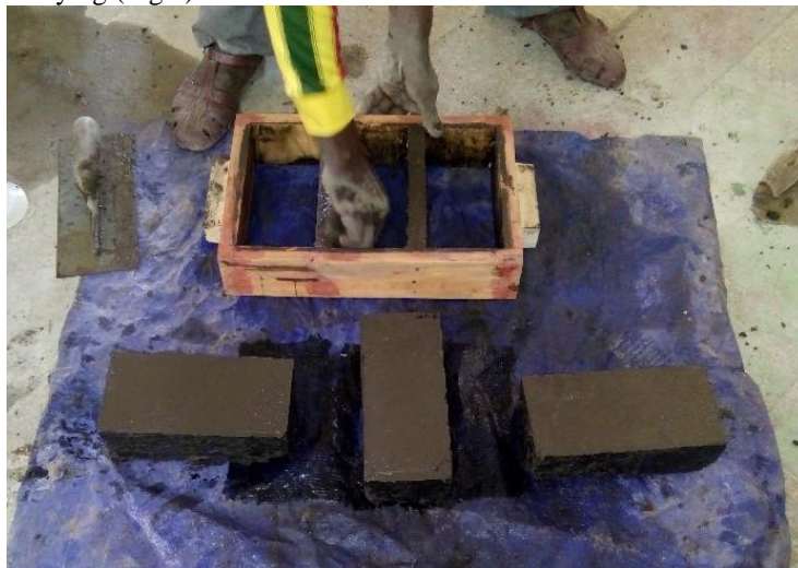
Figure 3. Mold used for casting adobe bricks
