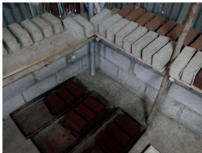
Figure 4. Adobe brick specimens under air curing
