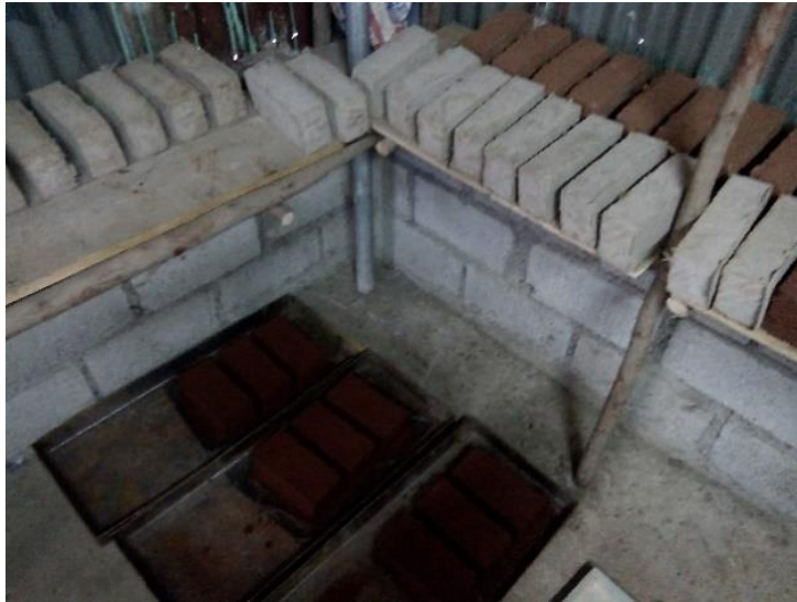
Figure 4. Adobe brick specimens under air curing
