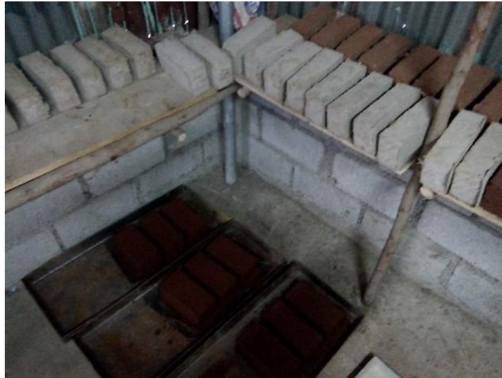
Figure 4. Adobe brick specimens under air curing
