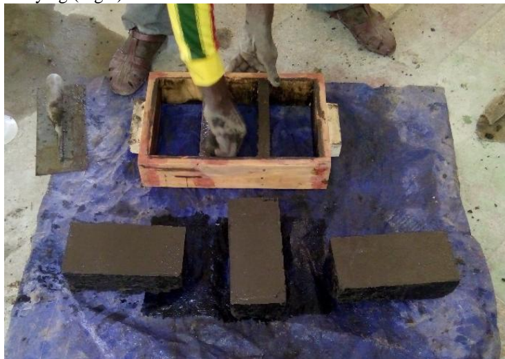
Figure 3. Mold used for casting adobe bricks
