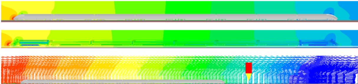
Figure 8: Aerodynamic resistance load distribution on ICE3 full-scaled train at yaw-angle  $\beta = 15^\circ$
